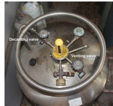
Decanting and vent valves
