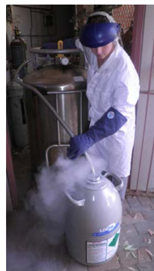
Decanting using PPE
