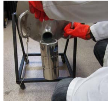
Decanting using a tipping stand
