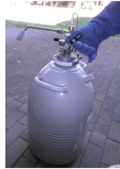
De-pressurising a Dewar
