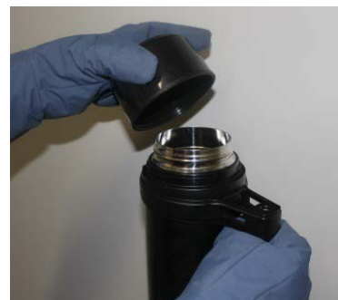
Loose fitting cap
