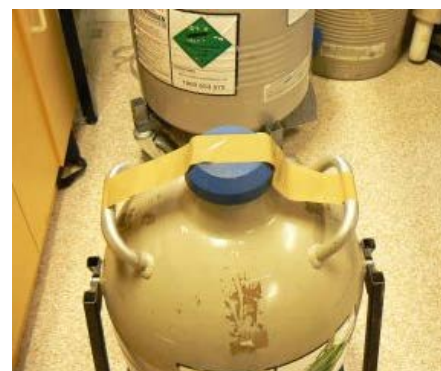
Dewar with cap taped in place
