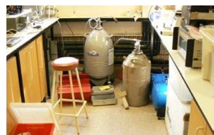
Incorrect storage of Dewars
