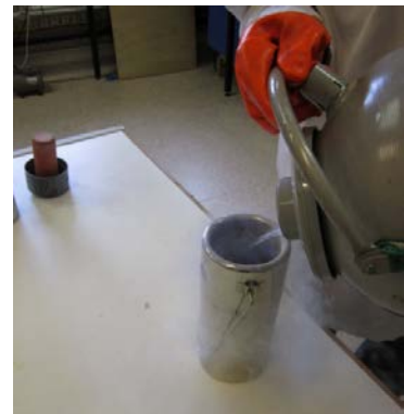
Decanting from small un-pressurised Dewar
