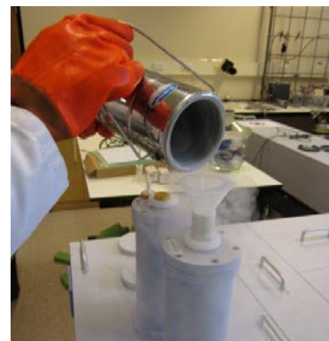
Decanting using a funnel
